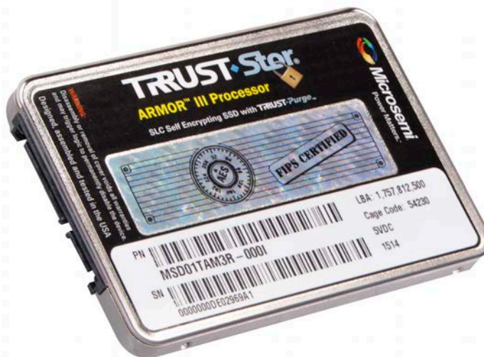
Figure 3 | TRUST-Stor solid-state devices, engineered specifically for defense applications, can be used in data recorders, ruggedized mobile systems, mobile man-packs, and ground vehicle applications.
