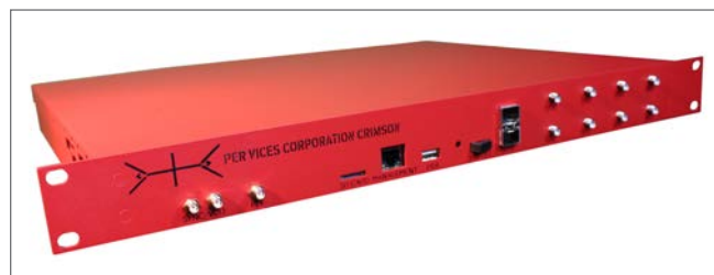
Figure 2 | The Crimson SDR has four independent receive and four independent transmit chains, each able to carry 322 MHz of RF bandwidth up to 6 GHz.
